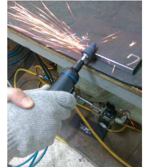
AT-7033DL(M) 1/4" (6MM) EXTENDED DIE GRINDER FREE SPEED: 22,000 RPM
